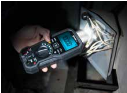
DM92 and DM93 feature powerful LED worklights
