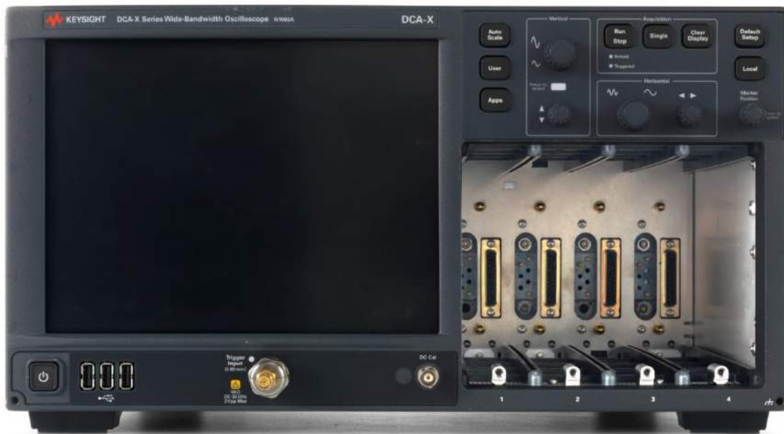
Figure 2: N1000A DCA-X mainframe (without option PTB)
