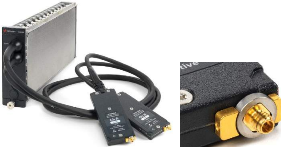
Figure 6: N1046A 100 GHz remote head module (with option 12F), 1.0 mm input connector detail
