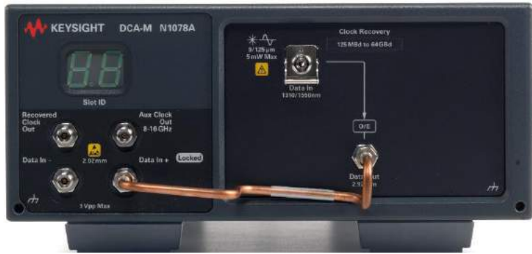
Figure 16: N1078A Single-mode optical/electrical clock recovery (with option S50)
