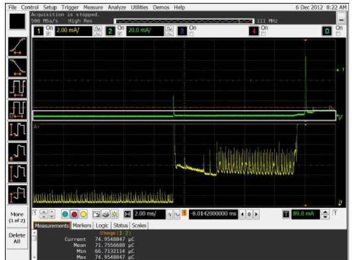
Figure 5. Infiniium oscilloscope coupled with the N2820A current probe provides the area under the curve measurement for accurate current consumption measurement.
