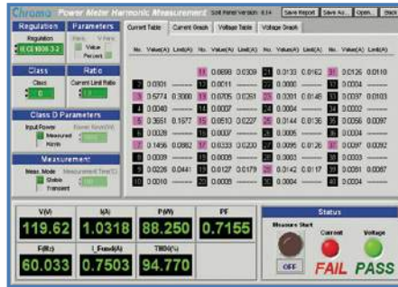
IEC 61000-3-2 Current Harmonics Test (Pre-compliance)
