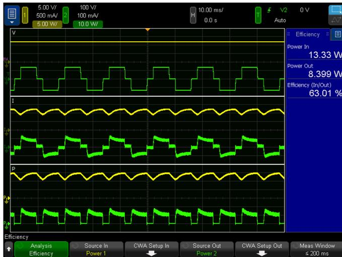
See real-time voltage, current and power on all channels simultaneously, with each parameter on its own grid (the default screen layout). Screen layout and functions are the same as a traditional oscilloscope.
