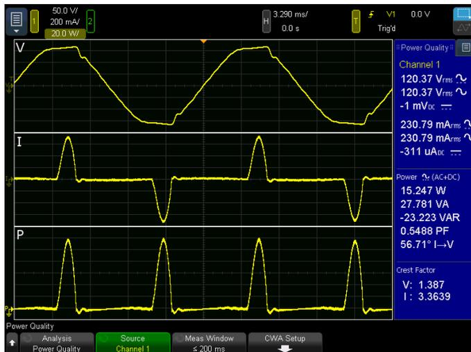
Press the [Analyze] key to view power quality measurements, shown in the blue Power Quality analysis panel. While displaying live power quality measurements, you can also view real-time voltage, current and power waveforms.
