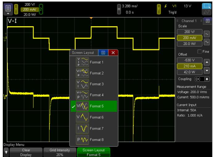
Choose from 8 different screen layouts of the voltage, current and power waveforms. Here, the Keysight IntegraVision power analyzer is displaying an enlarged view of voltage and current on the same grid to highlight the time relationship between voltage and current.
