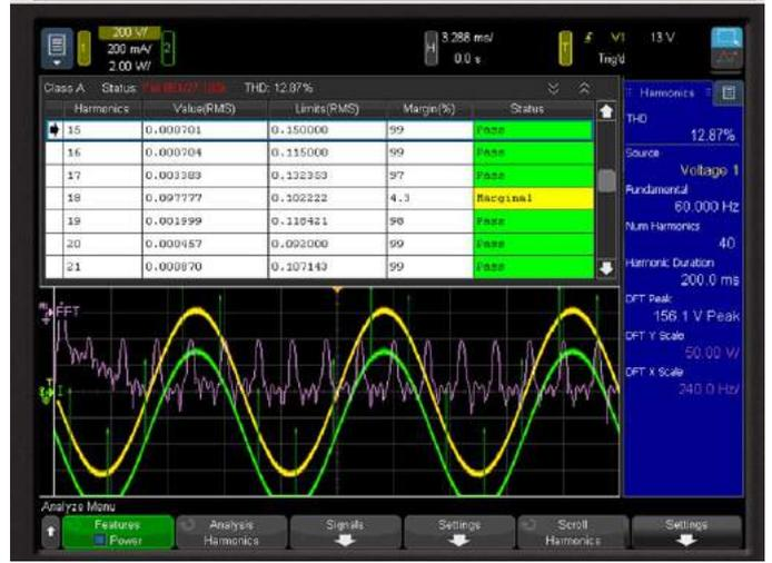
Quickly check harmonics with IEC 61000-3-2 limits (Classes A, B, C, and D)
