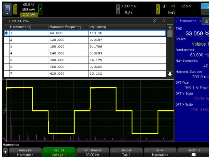
Perform harmonic analysis on voltage or current. Both the time domain waveform (yellow trace) and the harmonic table are simultaneously displayed.
