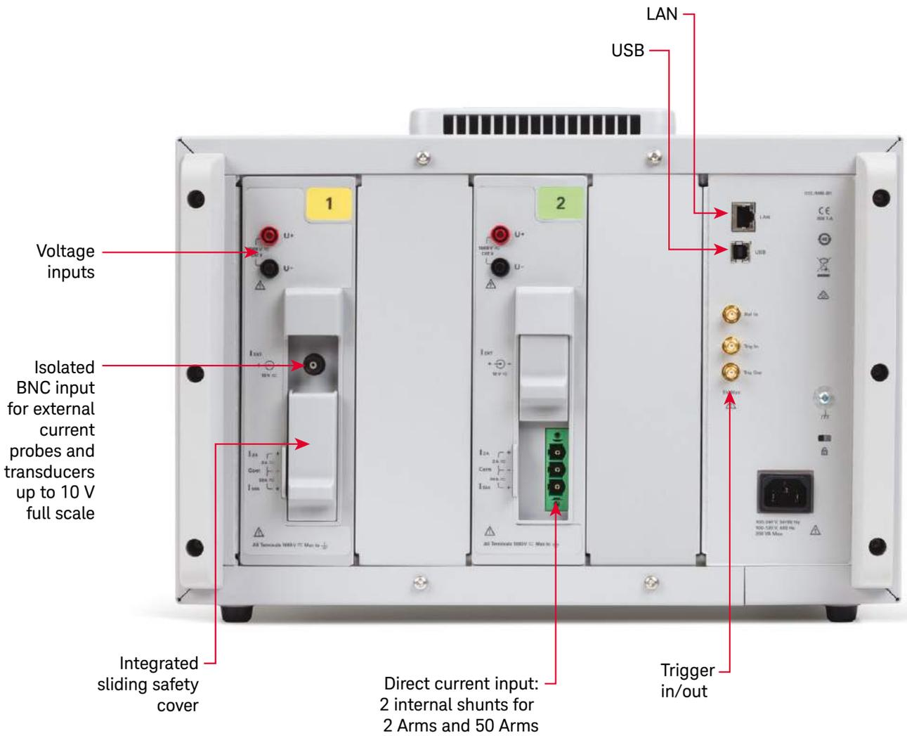
When measuring current with the direct current input, wiring to the DUT is connected on a removable connector, allowing you to quickly remove the wires for fast reconfiguration.
