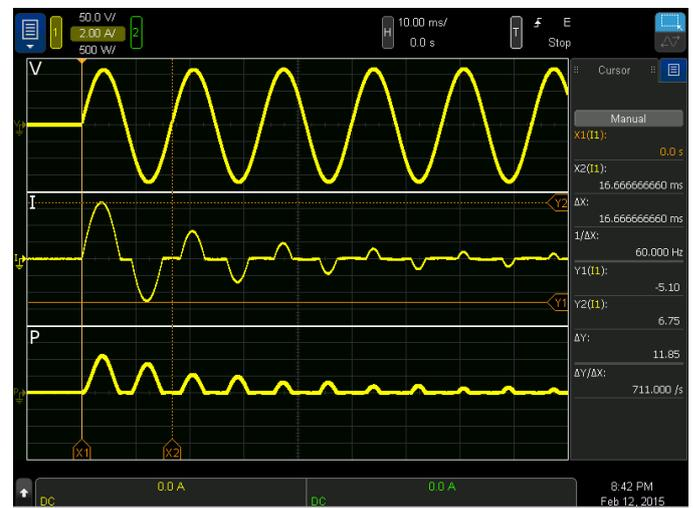
Use cursors to make common measurements, shown in the right side panel. Here, the Keysight IntegraVision power analyzer displays in-rush current (middle current trace) and power (bottom power trace) following an AC line input voltage turn-on (top voltage trace). The cursors show a peak of 6.75 A during the first cycle.
