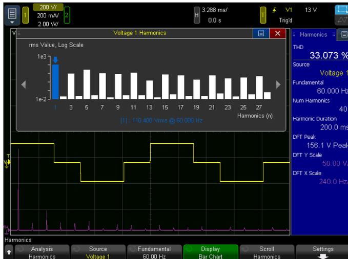
In addition to the harmonics table, simultaneously view a bar graph of the harmonic orders to visually identify high value harmonics.
