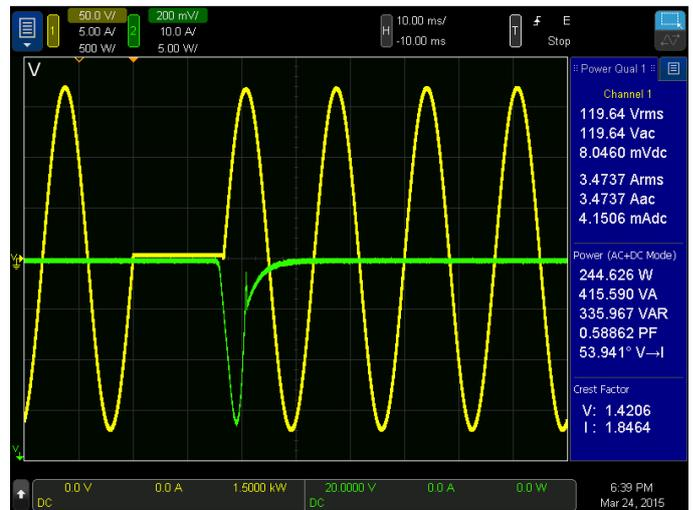
Use single-shot measurement mode to analyze power transients. Here the Keysight IntegraVision power analyzer displays an AC line voltage full-cycle dropout on one channel (yellow trace) and the corresponding response of a DC power supply output on the other channel (green trace). Thanks to single-shot measurement and visualization, you can easily see that the 20 V DC output drops about 0.6 V and then recovers in 10 ms.
