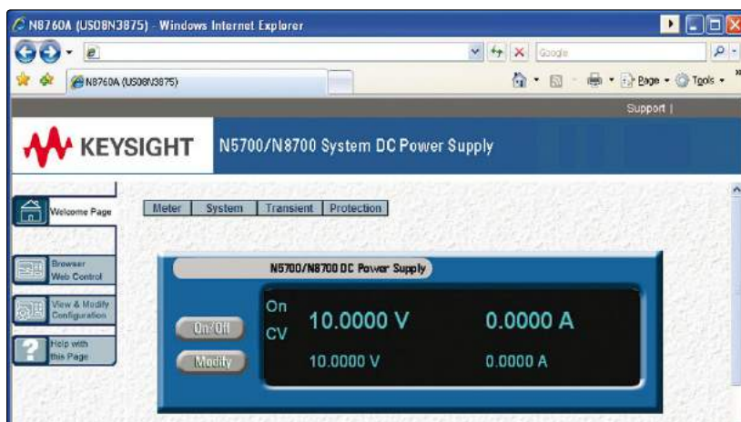
Figure 3. N8700 series web graphical user interface for remote access and control of the power supply
